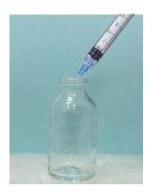
Wash glass bottle and syringe by clean water. Fill up the glass bottle with 3 ml of sample water.
