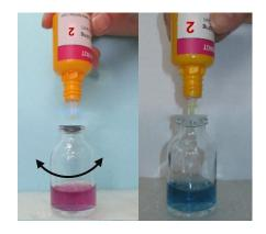
Slowly add the Reagent 2 dropwise, swirling to mix after each drop while counting number of drops until water turns purple. Continue until water changes to violet. Stop at the blue end point. A number of drops is a.
